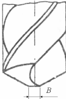
Fig.1. The contact model between drill and plane surface of work piece material.
